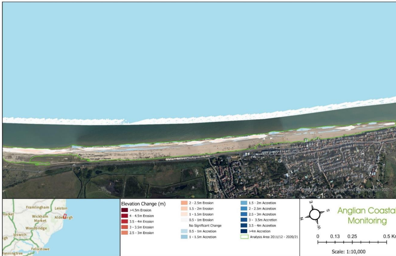
Plate 4.1.13 The difference in elevation from the LiDAR surveys in 2011 and 2021 for the Aldeburgh monitoring cell (Anglian Regional Coastal Monitoring Programme, 2022).
